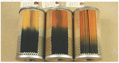
Sept. 24, 2015 — 3,243 miles on the filter; no fuel treatment. The filter was changed, and the fuel was treated with CarbonTreat™. Nov. 27, 2015 — 5,996 miles on filter; the first oil and filter change since the fuel was treated with CarbonTreat™. Feb. 18, 2016 — 5,879 miles on filter; the second oil and filter change since the fuel was treated with CarbonTreat™.
