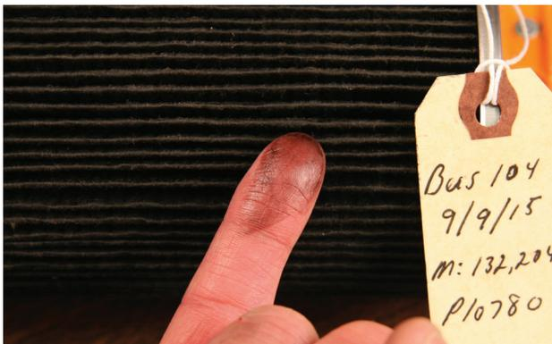
**Sept. 9, 2015 – no fuel treatment; 6000 miles on the filter.** Carbon and grit are evident in the filter, which indicates buildup in the fuel system. The filter was changed, and the fuel was treated with CarbonTreat™.
