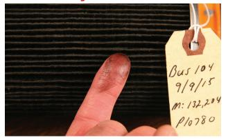
Sept. 9, 2015 – no fuel treatment; 6000 miles on the filter. Carbon and grit are evident in the filter, which indicates buildup in the fuel system. The filter was changed, and the fuel was treated with CarbonTreat™.
