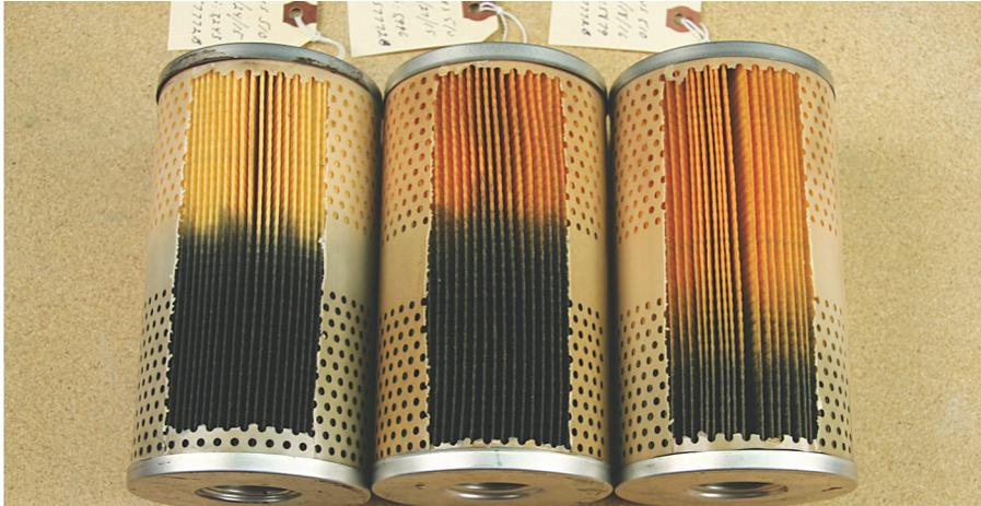
Sept. 24, 2015 – 3,243 miles on the filter; no fuel treatment. The filter was changed, and the fuel was treated with CarbonTreat™.
