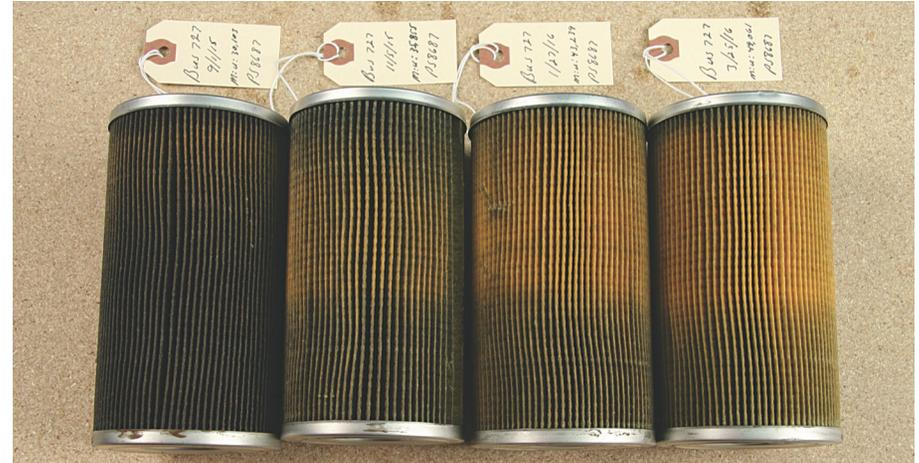
Sept. 1, 2015 – 6,000 miles on the filter; no fuel treatment. The filter was changed, and the fuel was treated with CarbonTreat™.
