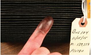
Nov. 15, 2015 — the first oil change since using CarbonTreat $^{\text{TM}}$ ; 6,130 miles on the filter.
