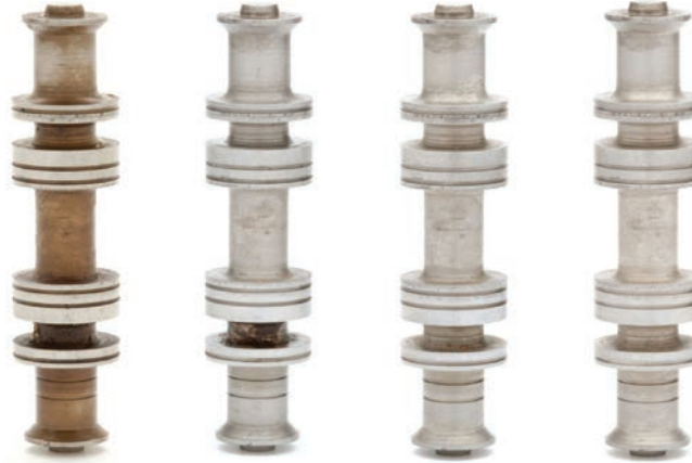
Valve clean up tea testing: Using the Extended Eaton-Vickers 35VQ Test, spools were placed in a bath and VarniClean was circulated across at 140 degrees F (60 degrees C). The spools were removed at the end of the test and rated 10 for clean using the CRC Rating Method. Photos were taken at 0, 1, 3 and 7 hours.
